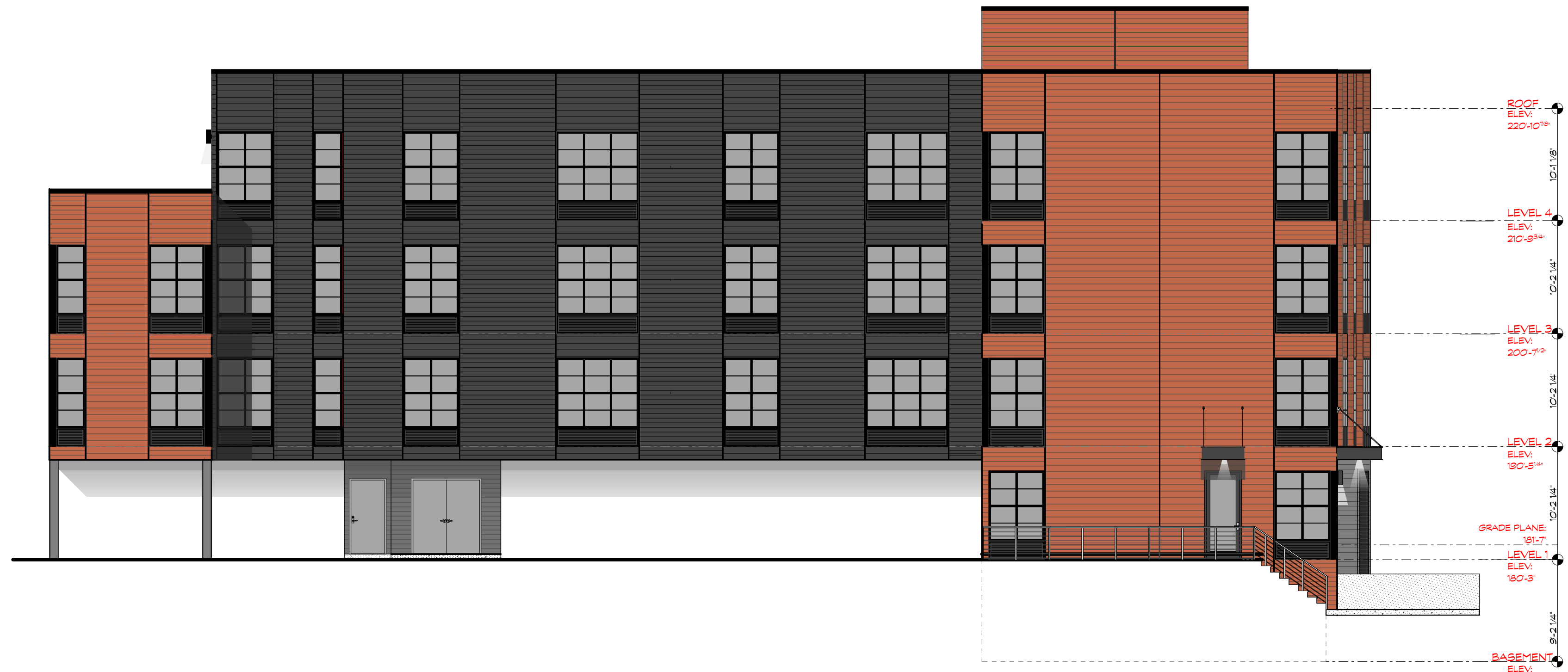
1 EAST ELEVATION - LAP SIDING SCALE: 1/8" = 1'-0"
