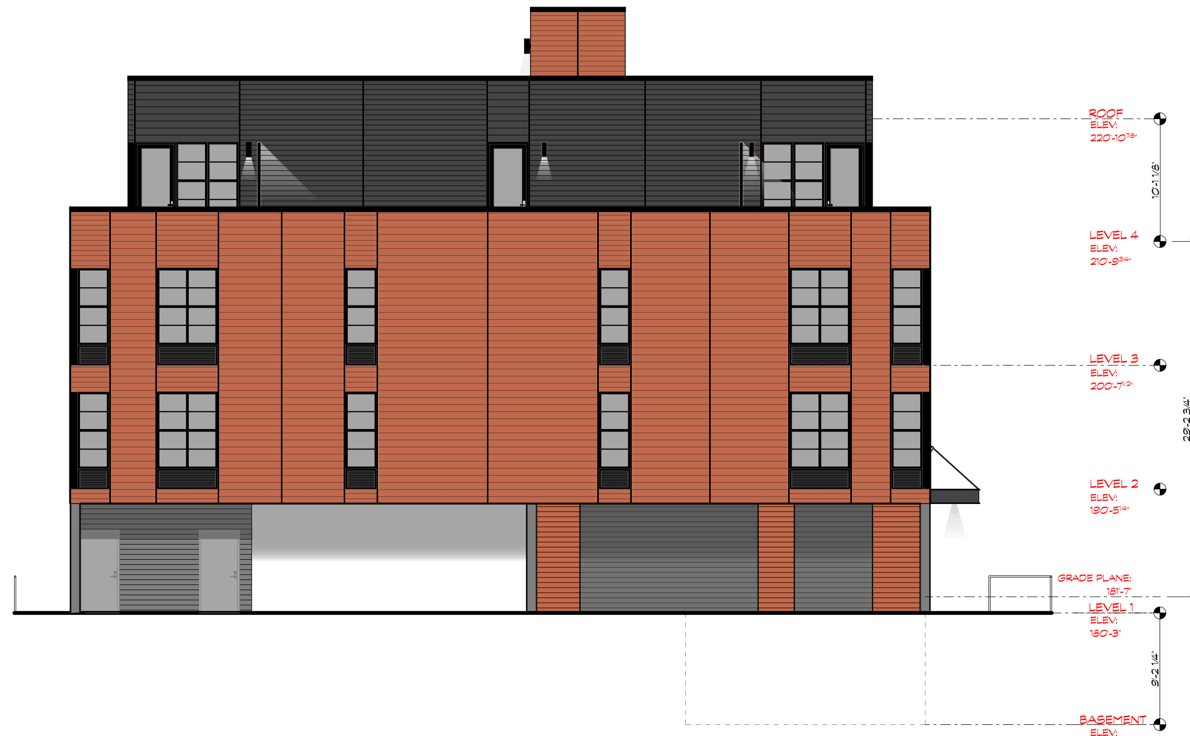
2 SOUTH ELEVATION - LAP SIDING SCALE: 1/8" = 1'-0"
